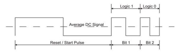
A 50/50-duty cycle will have an average DC signal resulting in a constant reference for the data slicer. Users should use pulse-width modulation to transmit data with logic 1's or 0's.
