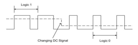
\*Only 50/50 duty cycle data is suitable for the T433 transmitter and R43305 receiver.
